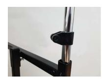
2. Remove Headrest from scooter and insert headrest rod into holes in the 16mm support tube. If this hole is too small for the headrest, it may have to be drilled to a larger diameter to suit.
