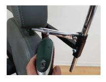
5. Move the Nylon clamp up or down and apply a small amount of vertical pressure on it before tightening up the clamp.
