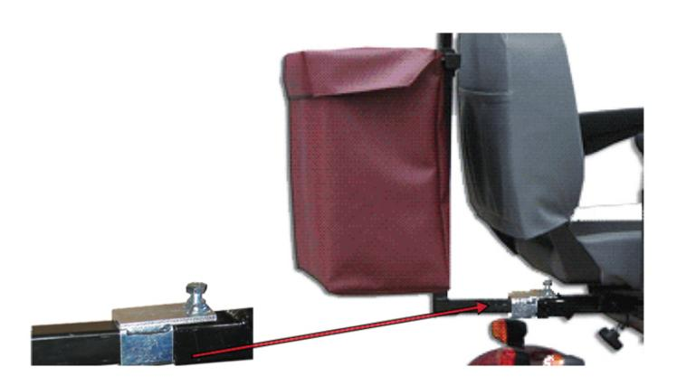
Slide Tow Bar Clamp onto "L" piece with the clamping tab facing the scooter.
